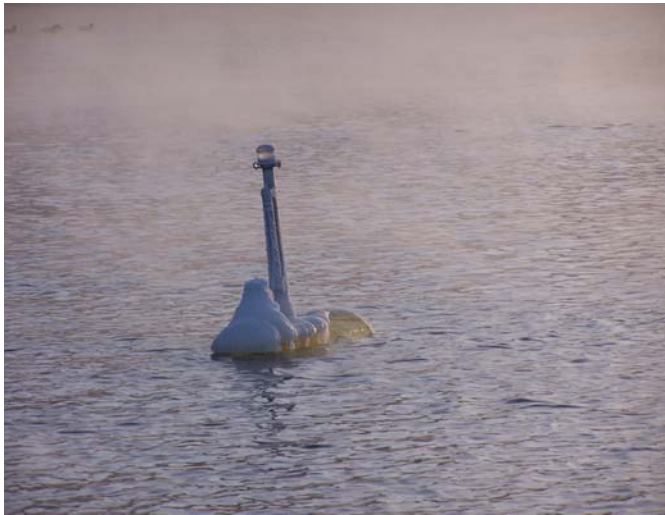
Fig. 4. Northwest Arm LOBO with heavy icing at -20 °C.
